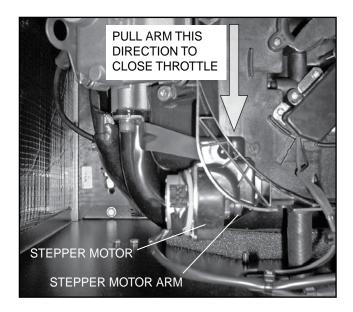
Figure 13. Throttle Positions 12-20 kW Units
